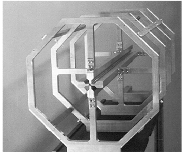
Fig. 1: The scaled 54 MHz cold model built at ITEP
