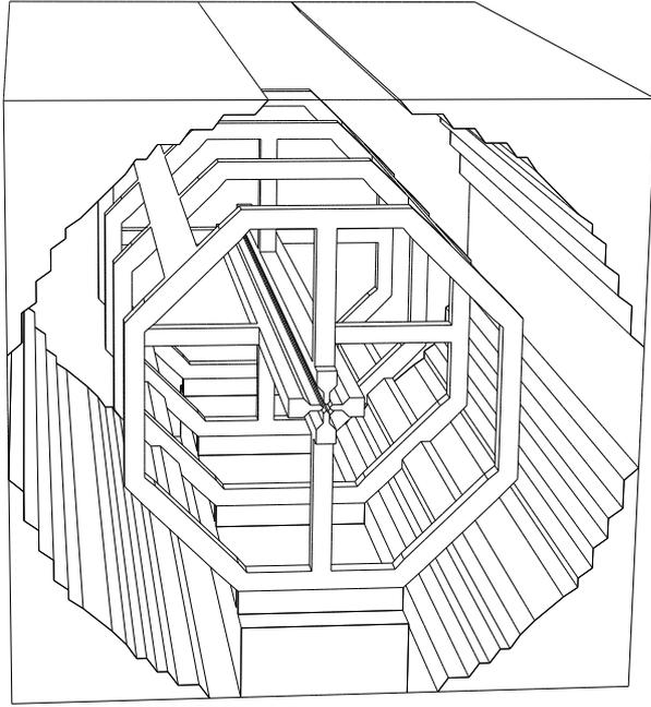
Fig. 2: MAFIA plot of the 54 MHz 3-cell RFQ
