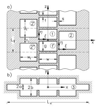
Figure 1: The biperiodic muffin–tin structure. a) Top–view b) transverse cut.
