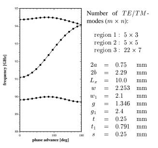
Figure 5: Dispersion relation of a side coupled accelerating structure with confluence in the  $\pi$ -mode.
