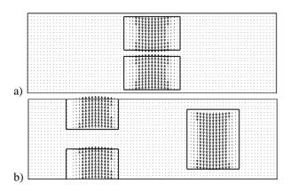
Figure 4: The 94 GHz  $\pi$ -mode field pattern in a structure a) without side coupling cells b) without main cells.
