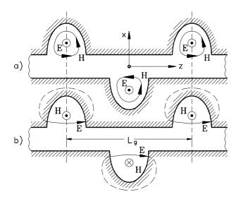
Figure 2: An alternating periodic structure with a) y-directed electric field, b) y-directed magnetic field.
