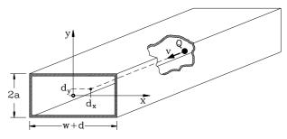
Figure 3: Point charge in a rectangular waveguide.
