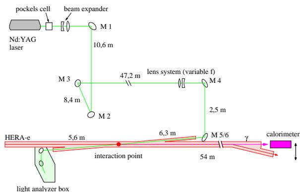
Figure 3: Layout of the longitudinal polarimeter
