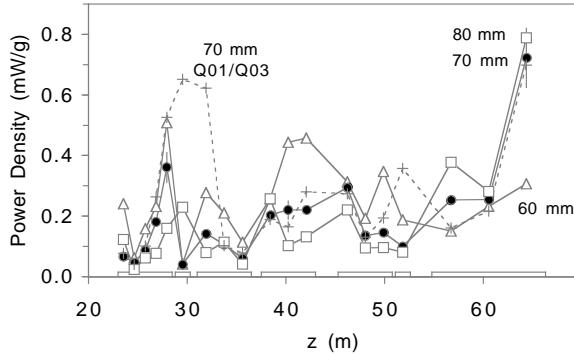
Figure 3:  $P_{max}$  vs  $z$  for main quadrupoles of three  $d_{coil}$  with 85 mm trim quadrupoles, and 70 mm main with 70 mm trim quadrupoles. The data are plotted at the  $z$  values for the 70 mm quadrupoles to ease comparison.
