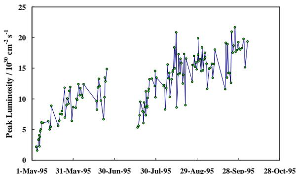
Figure 2 : Evolution of peak luminosity with bunch trains through the commissioning and energy scan periods.
