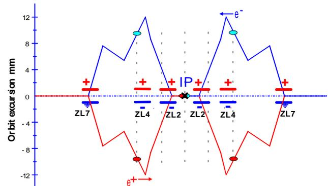
Figure 1 : The bunch train separation scheme for one experimental interaction point, with collisions at the IP.
