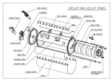
Fig. 1. Vacuum and helium tanks
