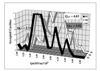
Fig. 5. LEP cavity performance vs. year of production
