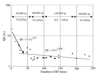
Figure 2. Quantum efficiency of Cs<sub>2</sub>Te cathodes as a function of RF hours. During the use of this cathode different RF field levels were applied as indicated.
