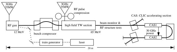
Figure 1. Schematic layout of CTF as it was in 1995
