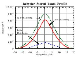
Figure 4. Stacking in the Recycler.
