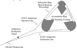
Figure 1. Antiproton Source Layout.
