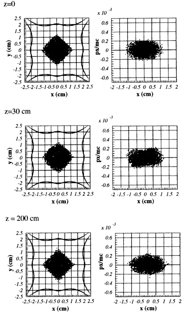
Fig. 2. Matching of the 150keV, 100mA,  $0.15 \pi \text{ cm mrad}$  proton beam in a uniform four-conductor quadrupole line with field gradient  $50 \text{ kV/cm}^2$ , duodecapole component  $-1.4 \text{ kV/cm}^6$  and frequency 270MHz.
