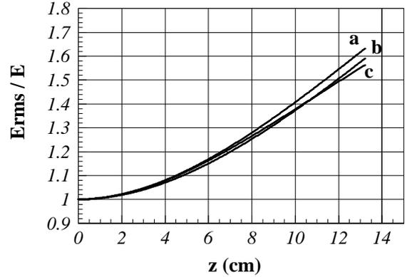
Fig. 5. Emittance growth of the beam with  $A/Z=5$ ,  $\beta = 1.9 \cdot 10^{-3}$ ,  $E = 1.5 \pi$  cm mrad for different values of initial beam radius: a)  $R = 2$ cm; b)  $R = 1$ cm; c)  $R = 0.5$  cm.
