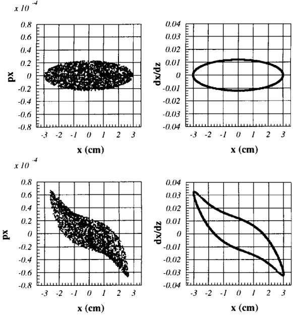
Fig. 3. Distortion of beam emittance shape due to aberration in einzel lens with parameter  $\delta = 1.5$ : numerical modeling (left) and calculated from formula (11).
