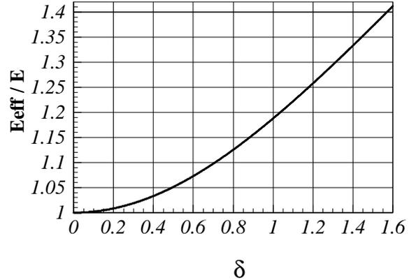
Fig. 4. Emittance growth due to aberration in einzel lens as a function of parameter  $\delta$ , calculated from formulas (11), (14).
