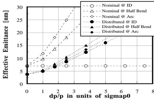
Fig. 2. Effective emittance versus rms momentum spread  $\sigma_p$ .
