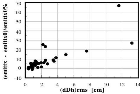
Fig. 5. Calculated emittance degradation versus different values of  $(\Delta D_h)_{rms}$  over many simulated machines.
