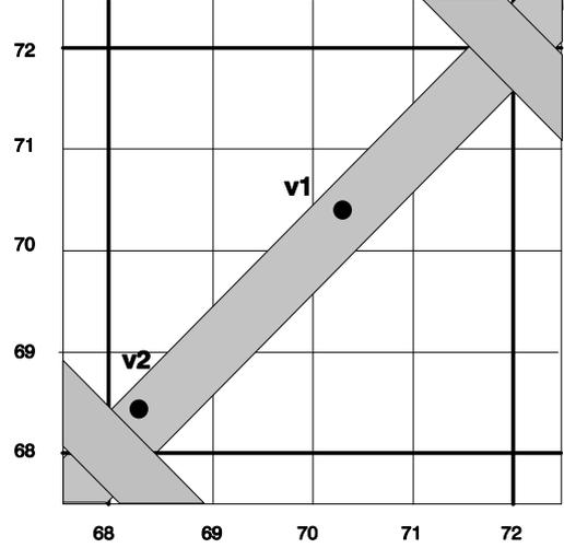
Figure 3: Systematic coupling resonances in LHC in  $Q_x, Q_y$  plane
