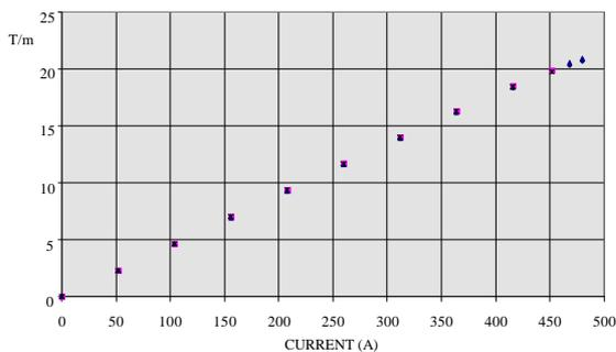
any magnetic length variation with excitation is transferred to the gradients. Figures 2-4 are the Hall probe measurements of the fields in the median plane with poly-fits to the data. The integrated sextupole component is extracted from the rot.coil measurements and calibration is done as described above. During the prototype measurements it was found that the dipole and sextupole must be corrected at higher excitations.
