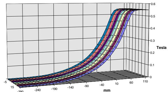
Fig. 6 DIPOLE MEDIAN FIELD (0.5 T)
