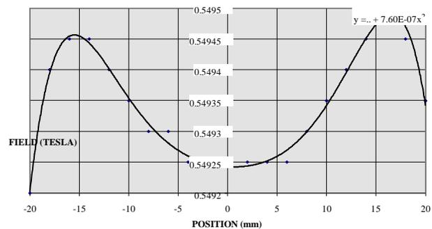
Fig. 7 DIPOLE MEDIAN PLANE FIELD (1.5 T)
