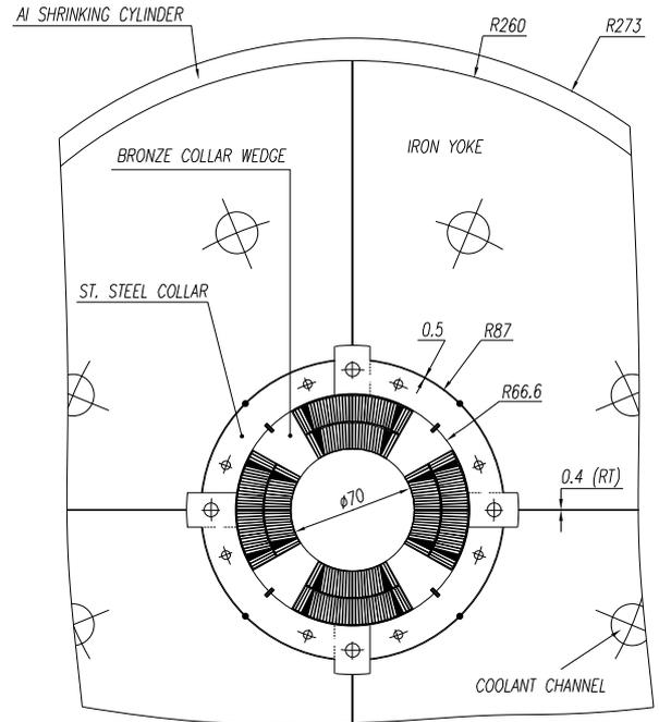
Figure 1: Schematic cross section of the Nb<sub>3</sub>Sn quadrupole.
