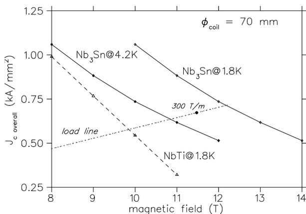
Figure 2: Coil  $J_c$  for our Nb<sub>3</sub>Sn and for NbTi and magnet load line.
