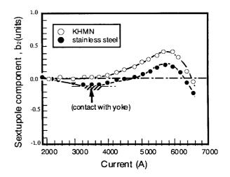
Fig. 5 Change in sextupole error component with current in dipole small magnets with KHMN and stainless steel collars (SSCL)
