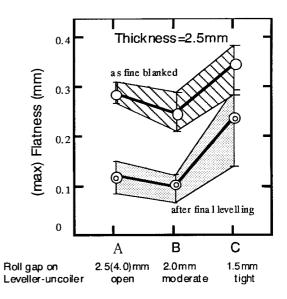
Fig. 3 Flatness of fine-blanked KHMN collars before and after final correction levelling
