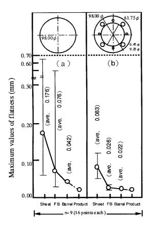
Fig. 4 Flatness measurement at each process of fine-blanking (FB) of 6.35 mm thick EFE sheets for (yoke) products
