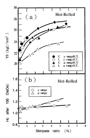
Fig.2 Relations between yield stress (YS) or coercive force (Hc) and skin pass ratio of 6.3 mm thick hot-rolled EFE heat treated at  $\gamma$  or  $\alpha$  - range temperatures (without annealing).
