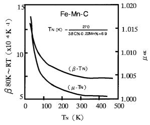
Fig. 1 Relation between thermal expansivity,  $\beta$  or magnetic permiability,  $\mu$ , and the Néel temperature, TN, that is formulated by the equation herein.
