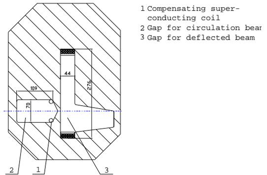
Figure 6: Cross-section of the second section of the Lambertson magnet
