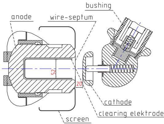
Figure 2: Schematic drawing of the electrostatic septum
