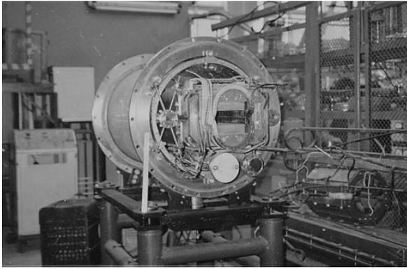
Figure 7: View of the wide aperture dipole magnet
