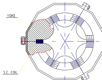
Figure 1: Cross-section of the sextupole superconducting extraction lens
