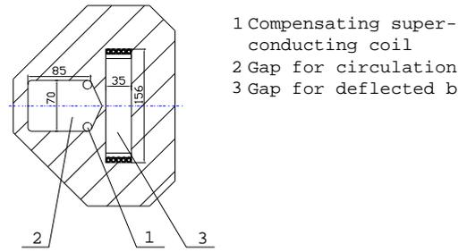
Figure 5: Cross-section of the first section of the Lambertson magnet
