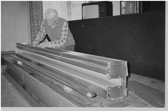
Figure 3: View of the ES anode and cathode
