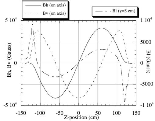
Fig. 5 Calculated magnetic field distribution in helical dipole magnet.
