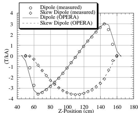
Fig. 2 Dipole component of the model magnet.
