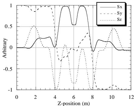
Fig. 8 Spin motion in magnetic field created by 3D analysis.
