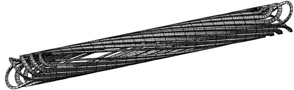
Fig. 1 The model of helical dipole magnet.
