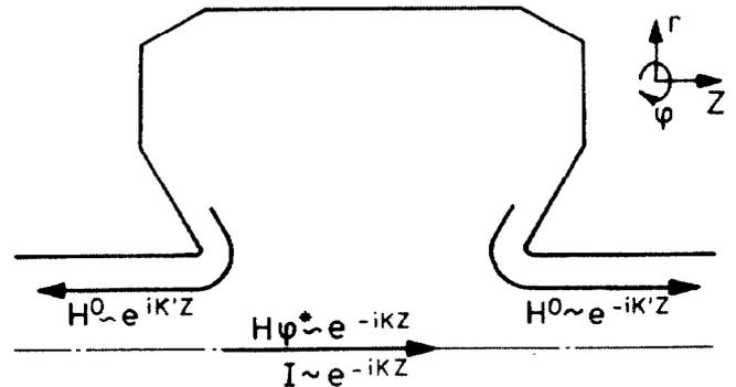
Figure 1: Longitudinal dependence of exciting current and magnetic field components.
