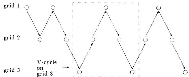
Figure 4: FMG-method with three grids and two V-cycles on each grid. Grid 1 is the coarsest grid.
