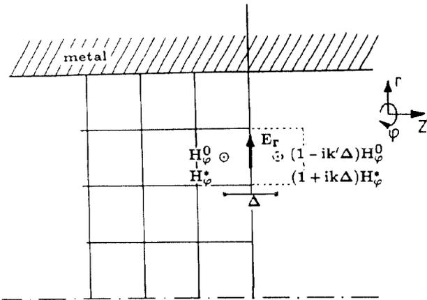
Figure 2: Use of the open boundary condition at the grid boundary in the tube to the right side of the cavity.
