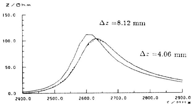
Figure 8: Comparison of real part of the impedance by direct solution on grid with  $\Delta z = 8.12$  mm and by 2-grid-MG-solution respectively direct solution on grid with  $\Delta z = 4.06$  mm (cut-off = 2295 MHz).
