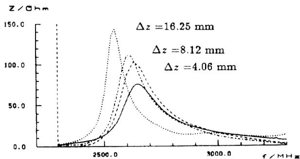
Figure 7: Real part of the impedance above cut-off (= 2295 MHz) calculated by URMEL-I with direct solution method and stepsizes  $\Delta z = 4.06, 8.12, 16.25$  mm and impedance by analytical solution with Henke's code.
