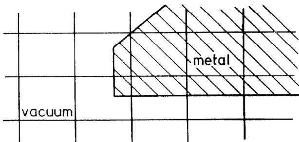
Figure 3: Partially filled grid cells.
