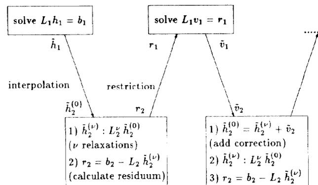
Figure 5: FMG-method on two grids.
