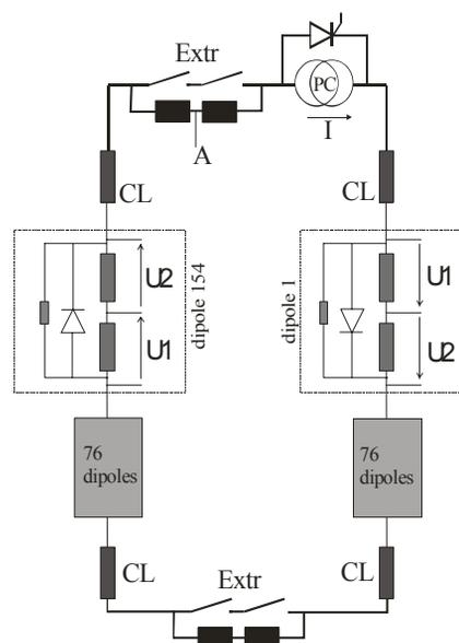
Figure 1: Schematic view of a dipole circuit of one octant of the LHC. Note that only the first and last dipoles of the circuit are shown in more detail. The system is grounded at point A by a circuit of resistances and a fuse. Each dipole is shunted by a 100  $\Omega$  damping resistance to reduce voltage oscillations after opening of the extraction switches. CL=Current Lead
