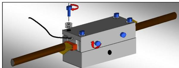
Figure 1: Design of an oven for resistive soldering
