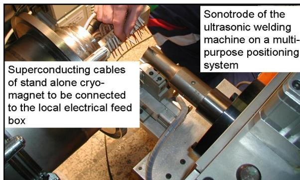
Figure 2: Ultrasonic welding in the special IC
