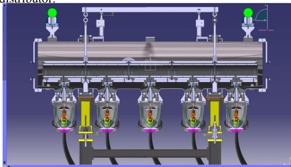
Figure 2: BIDIS assembly cross section, showing the 5 magnets inside the vacuum vessel and the associated feedthroughs and connection boxes below the tank.
