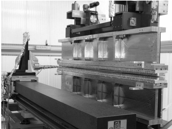
Figure 1: The magnetic field measurement bench with one of the ACCEL undulator sections under test at ENEA Frascati Laboratories.
