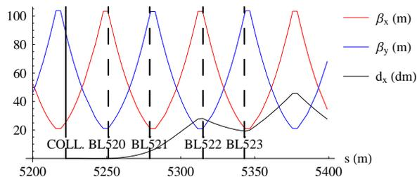
Figure 1: The  $\beta$ -functions of the SPS just downstream of the collimator together with the locally generated dispersion  $d_x$  from the collimator. The locations of the BLMs and the collimator are indicated by vertical lines.
