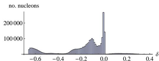
Figure 6: The distribution of  $\delta$  of all ion fragments coming out of the collimator. The heights of the bars show the number of nucleons belonging to ions having  $\delta$  within a certain interval.
