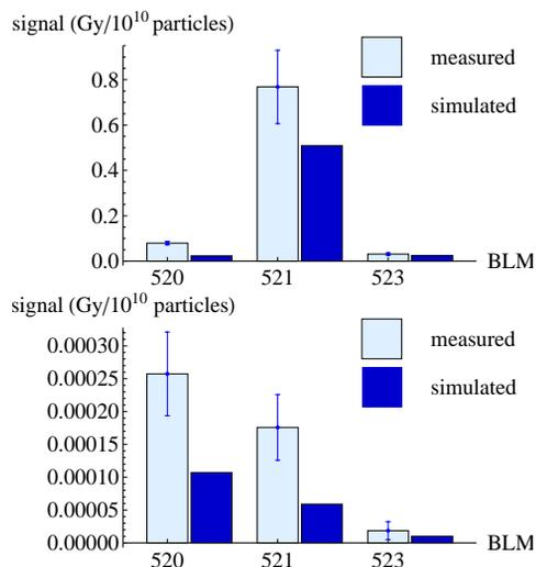
Figure 5: Average measured ion (top) and proton (bottom) loss map from the BLMs downstream of the collimator compared with simulations normalized to  $10^{10}$  lost particles. The standard deviation between different measurements is indicated.
