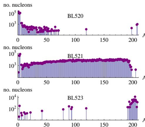
Figure 7: The  $A$  distribution of ion fragments lost within 15 m upstream of each BLM. The heights of the bars show the number of nucleons from ions having a certain  $A$ .
