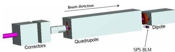
Figure 3: The geometry as implemented in FLUKA around the monitor BL520, which is located around 30 m downstream of the collimator in the SPS.
