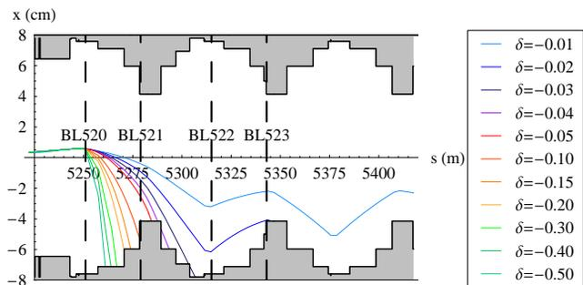
Figure 2: Dispersive orbits of fragmented ions produced in one of the collimator jaws, shown together with the aperture. The vertical dashed lines indicate the location of the four BLMs closest downstream.
