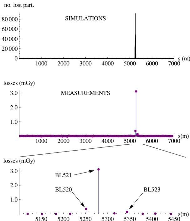
Figure 4: Example of simulated ICOSIM (top) and measured (middle)  $^{208}\text{Pb}^{82+}$  ion loss map for the whole SPS ring. The bottom part shows a closeup of the loss peak in the measurements, with the names of the BLMs with the highest signals indicated. The simulated losses were binned in 5 m intervals. The collimator is located at  $s = 5222$  m, just upstream of the large loss peak.
