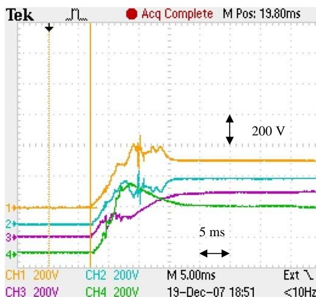
Figure 2: Voltages across the opening switches for an 11 kA quench.
