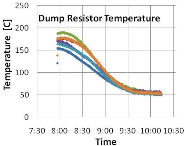
Figure 4: Cool down of the dump resistors.
