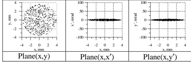
Figure 1: K-V type distribution in various phase planes.  $Sgn(B_{ECR}B_0) = 1$
