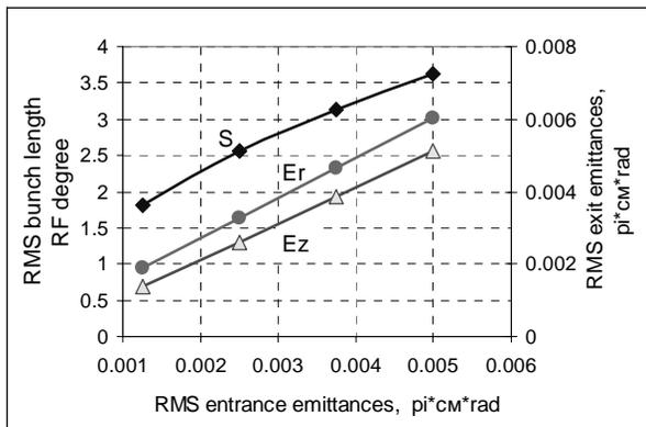
Figure 3: Horizontal ( $E_r$ ) and vertical ( $E_z$ ) RMS emittances and RMS bunch lengthening ( $S$ ) vs  $\epsilon_{rms} \cdot \text{Sgn}(B_{ECR}B_0) = 1$
