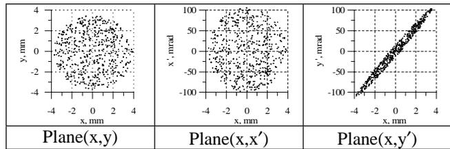
Figure 2: K-V type distribution in various phase planes.  $Sgn(B_{ECR}B_0) = -1$
