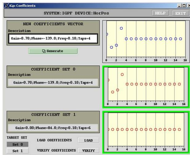
Figure 2: FIR filter coefficient set EPICS panel.
