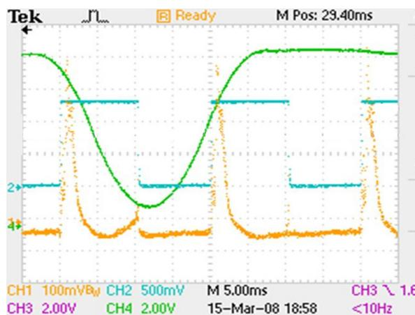
Figure 2. First operation of the MICE target with beam. The signals shown are the target trajectory (arb. units, green), circulating intensity in ISIS (blue) and the ISIS beamloss sum signal (yellow). The beamloss signal shows a rise at ~6-10ms as the MICE target is inserted. No interference is seen with subsequent ISIS pulses.
