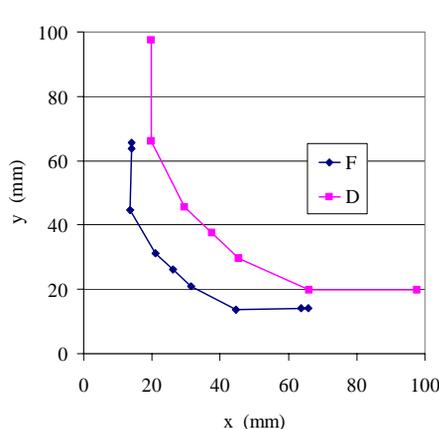
Figure 1: Pole profile for F and D magnets.
