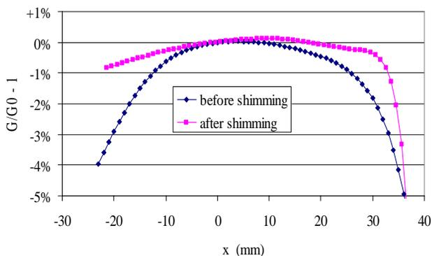
Figure 7: Relative integrated gradient quality of the D magnet before and after shimming; the D's magnetic centre is at -22.6 mm; the F magnet is un-powered.
