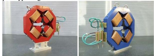
Figure 2: The prototype magnets (F left, D right).
