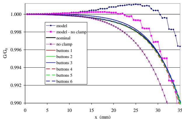
Figure 4: Normalised integrated gradient vs transverse ( $x$ ) position (from coil rotational centre) for the F (top) and D (bottom) magnets. The model predictions are shown with blue and purple lines in each figure.
