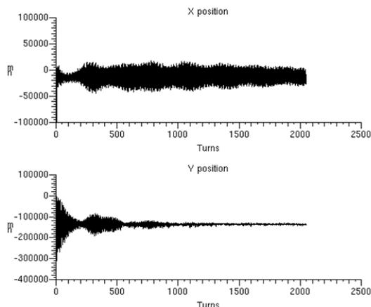
Figure 7: Turn-by-turn BPM measurement of kick following fine tuning of injection kickers. Maximum kicks are  $\pm 30 \mu\text{m}$  and  $\pm 140 \mu\text{m}$  in horizontal and vertical planes respectively.
