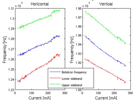
Figure 4: Drift in betatron tune and sidebands
