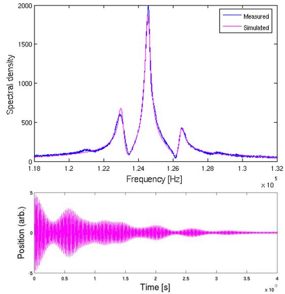
Figure 5: Measured and reconstructed tune profile (top) and reconstructed turn-by-turn trace (bottom).
