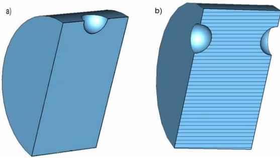
Figure 3: Pillbox cavity with top a) and side b) dents.
