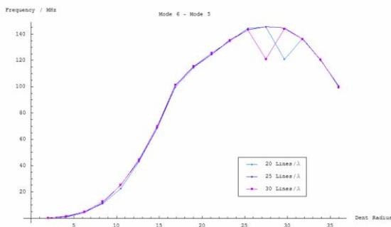
Figure 5: Mode degeneracy for a pillbox cavity with dent at the sides.
