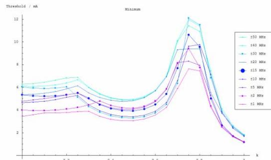
Figure 2: Minimum threshold for a multi-cavity system for HOMs with different degeneracy.
