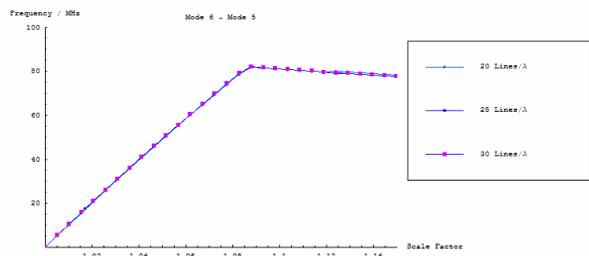
Figure 8: Mode degeneracy for a pillbox cavity extended in one dimension
