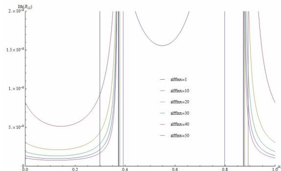
Figure 12: BBU threshold as a function of  $\alpha$  and  $\mu$ .
