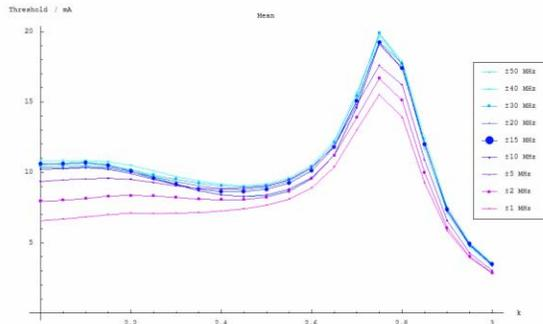
Figure 1: Average threshold for a multi-cavity system for HOMs with different degeneracy.
