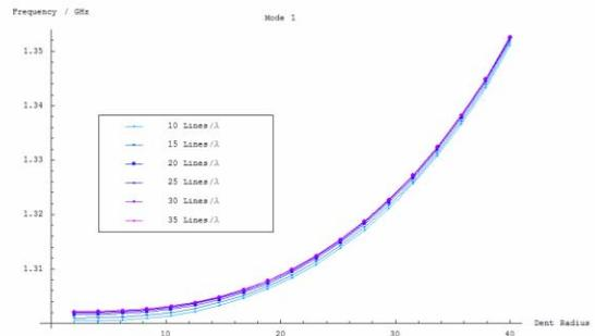
Figure 7: Change in fundamental frequency for a pillbox cavity with a dent at the sides.
