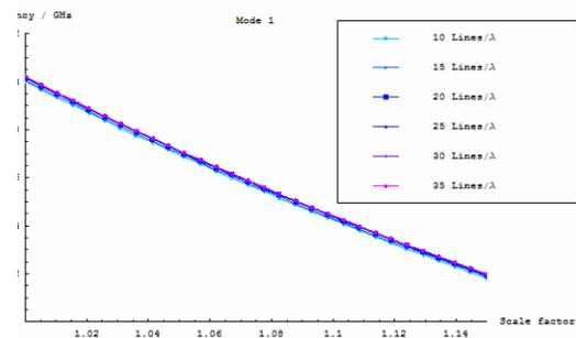
Figure 9: Change in fundamental frequency for a pillbox cavity extended in one dimension
