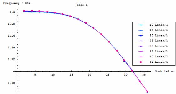
Figure 6: Change in fundamental frequency for a pillbox cavity with a dent at the top.
