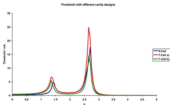
Figure 11: BBU Threshold for different transition from the cavity to a larger beam pipe for a TESLA type cavity.
