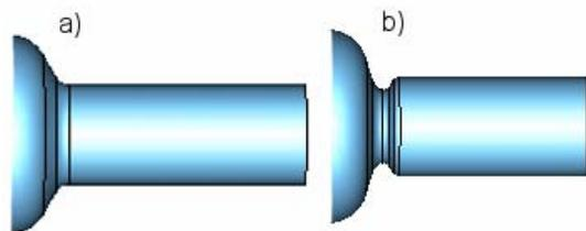
Figure 10: Transition from the cavity to a larger beam pipe for a TESLA type cavity.
