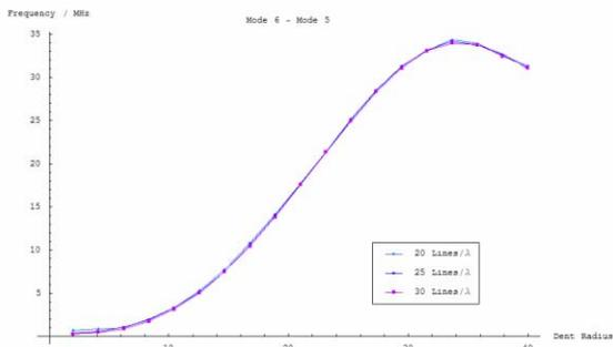
Figure 4: Mode degeneracy for a pillbox cavity with dent at the top.
