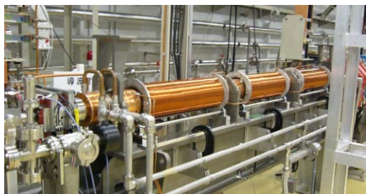
Fig. 5: solenoid coils covering the first accelerating structure.
