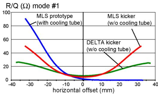
Figure 5: R/Q-factors of the first resonant mode in the MLS and DELTA kicker respectively computed at different horizontal offsets. Asymmetric fields can be induced by implementing a cooling tube.
