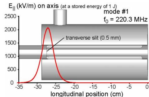
Figure 4: Computed on axis electric field of mode #1.
