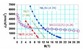
Fig 1: Critical current as a function of field for NbTi, Nb<sub>3</sub>Sn and BSCCO 2212.
