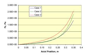
Fig 5: Axial force density along magnet length for each case at the radius where the force density is maximal.
