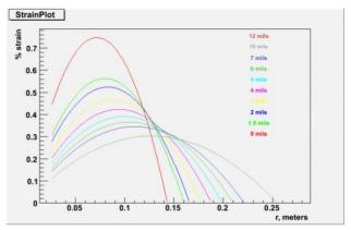
Fig 3: Tensile strain on the HTS conductor as a function of radial position for various thicknesses of stainless steel interleaving in a 40 Tesla solenoid.
