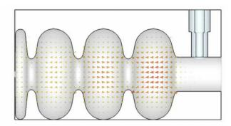
Figure 1: Profile of the electric field in the SCRF gun as calculated with the CST code.
