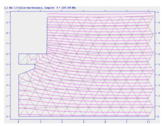
Figure 5: SUPERFISH sketch of the field lines near the retracted photocathode with visor.
