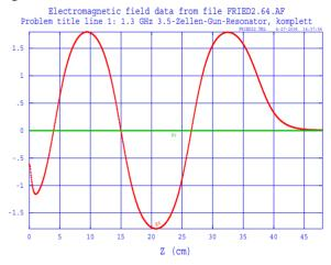
Figure 2: Distribution of the RF accelerating electrical field along the cavity axis as calculated with the Superfish code.
