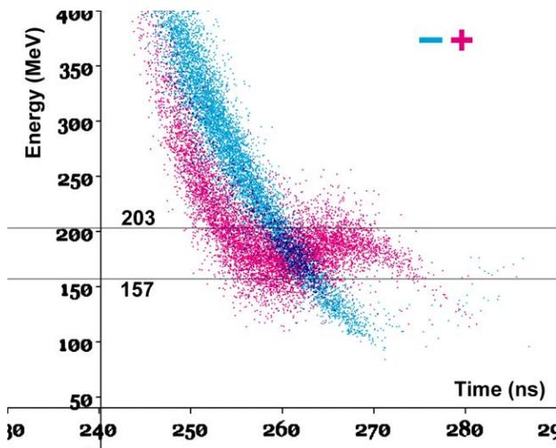
Figure 4: Longitudinal phase space of  $\mu^+$  (pink) and  $\mu^-$  (blue) leaving the phase rotator for the 8 GeV case.
