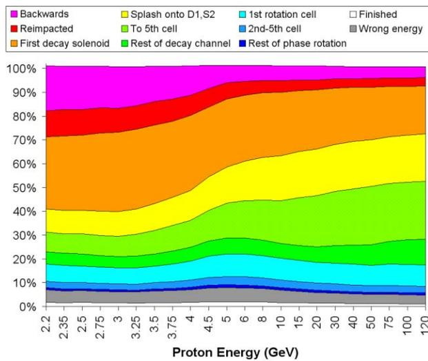
Figure 5: Loss types as a fraction of particle count. The sum is slightly more than 100% due to decays such as  $K^+ \rightarrow \pi^+ \pi^+ \pi^-$ .
