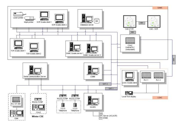
Figure 3: CSAM hardware architecture.
