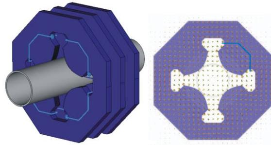
Figure 3: Compact triplet (left), Field distribution at a cross-section of one quadrupole (CST EM STUDIO<sup>TM</sup>).
