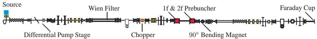
Figure 4: Offline Test stand of the Polarized Injector.
