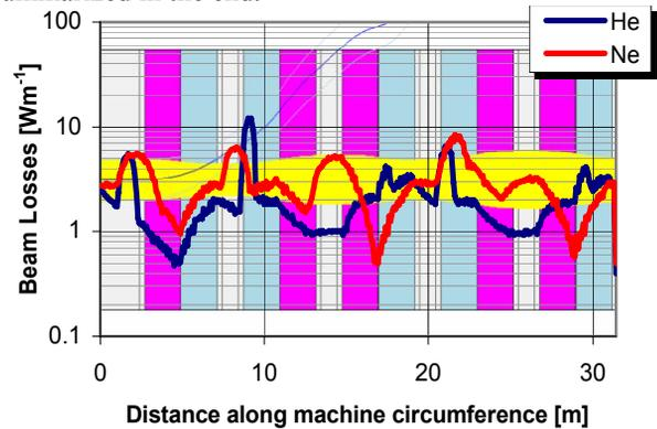
Figure 4: Loss distribution in terms of power deposition along one super cell of the PS machine for the case of  ${}^6\text{He}$  (blue) and  ${}^{18}\text{Ne}$  (red). The red and blue blocks indicate the position of the PS dipoles.
