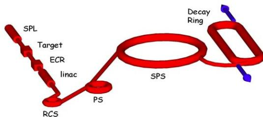
Figure 1: Schematic layout of the beta-beam complex.
