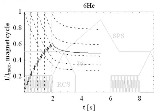
Figure 2: Cycle of the Beta-beam complex accelerating  ${}^6\text{He}$ . For illustration purposes the single bunch intensities (dashed) are indicated for the 1st, 5th, 10th, 15th and 20th bunch.
