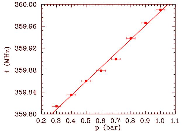
Figure 4: Measured frequency as function of the external pressure at T=77 K.
