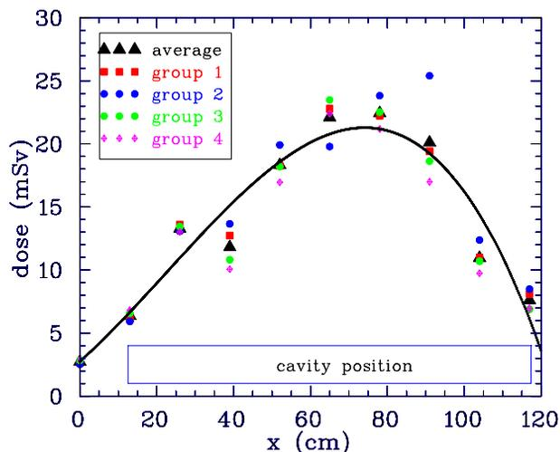
Figure 8: Measured X-ray distribution along the cavity.
