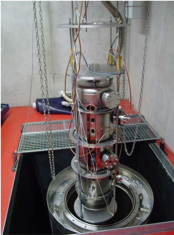
Figure 2: The superconducting CH-cavity ready for the first cold test in the vertical cryostat.
