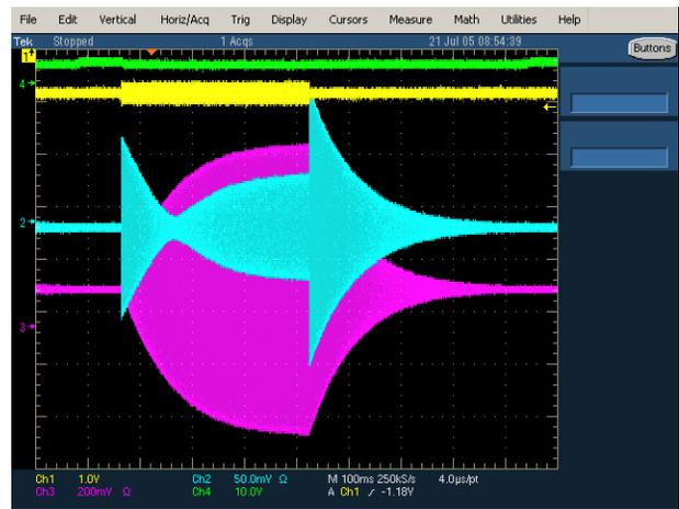
Figure 5: RF signals of the CH-cavity at low fields: Reflected signal (green), pickup signal (magenta) and forwarded signal (yellow). The time scale is 100 ms per division.
