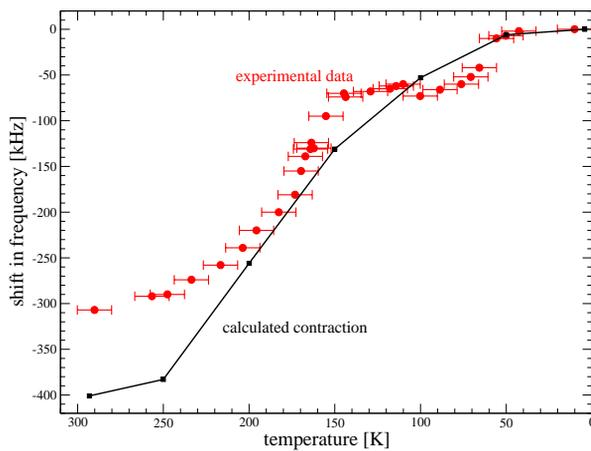
Figure 3: Measured frequency shift during the cooldown. The solid line represents the simulated frequency shift due to the contraction of the material.
