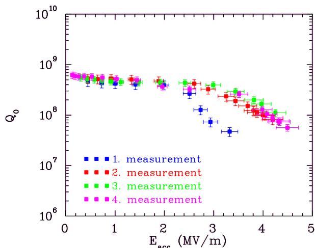
Figure 6: Measured unloaded Q-value  $Q_0$  as function of the accelerating gradient  $E_a$ . For the gradient definition a length of  $8.5\beta\lambda$  has been used.
