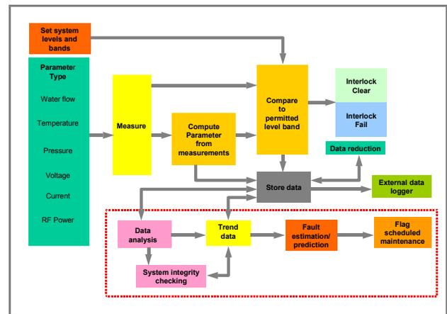
Figure 1: IOT Amplifier Basic Control Scheme
