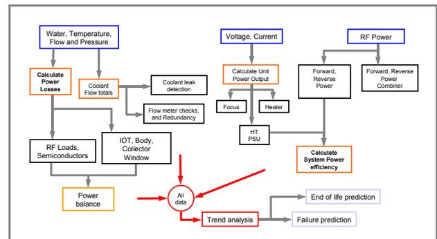
Figure 2: Measurements and System Calculations
