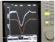
Figure 8: White (top): Recovered signal from the Single-Shot Fiber Scope Red (bottom): Original signal produced by the Impulse Signal Generator
