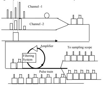
Figure 1: Single-shot fiber scope system
