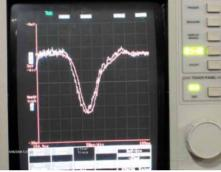
Figure 9: White: Recovered signal Red: Original signal Time scale: 50ps/div.
