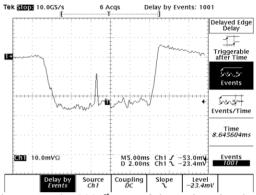
Figure 7: The 1001<sup>st</sup> turn of the gating signal with a captured single-shot signal.
