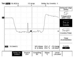
Figure 4: The first turn of the gating signal with a captured single-shot signal
