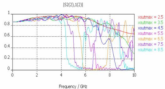
Figure 5 S<sub>21</sub> of meander line
