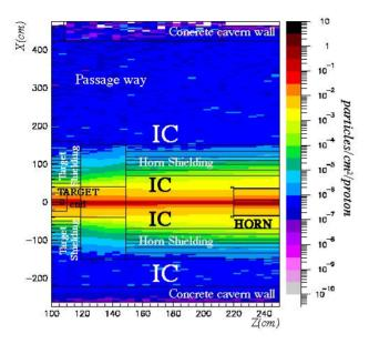
Figure 5: Fluence of all charged particles in the area intended for the ionization chambers location (IC).
