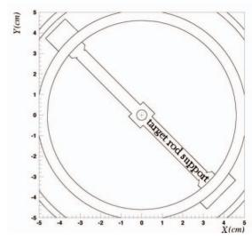
Figure 3: Transversal section of the target tube including the graphite supports of the target rods as described in FLUKA code
