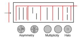
Figure 1: Schematic representation of the TBID: the disks (black) represent secondary emission titanium foil, the red lines represent electrodes.
