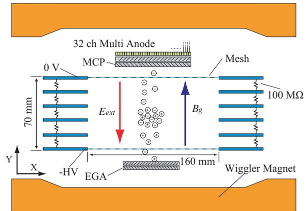
Figure 1: Cross section view of the prototype.
