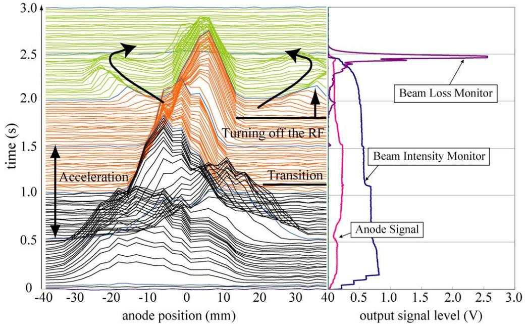
Figure 2: Mountain view of the obtained profiles for the ion collection mode (left). Raw signals from the MCP central anode (-1.25 mm from the center), a beam intensity monitor, and a beam loss monitor are also shown (right).
