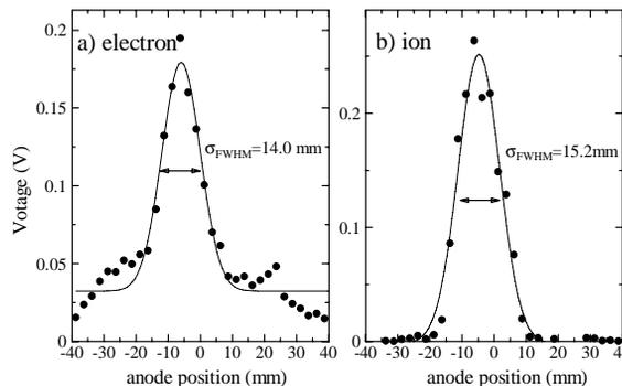
Figure 3: Typical beam profiles obtained at just before the transition energy, 1 s after the injection, for electron collection mode a) and for ion collection mode b). The solid lines are the fitted results.
