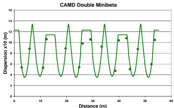
Figure 4: The calculated dispersion function x10 compared with the measured values.
