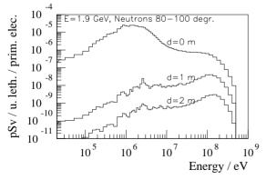
Figure 1: Neutron spectra thick from Cu target at  $90^{\circ}$
