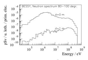
Figure 4: Neutron spectra at  $90^{\circ}$ , thin Fe target
