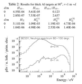
Figure 3: Neutron spectra at 90<sup>0</sup>, Al-Target
