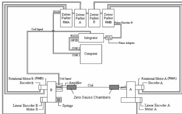
Figure 1: Schematic drawing of rotating coil system
