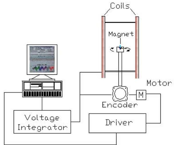
Figure 4: Schematic representation of the magnetic blocks characterization system
