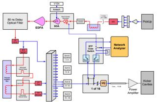
Figure 2: Block diagram of the low level electronics. Red indicates fiber optic, blue is coax. EDFA=erbium doped fiber amplifier, SOA=semiconductor optical amplifier.
