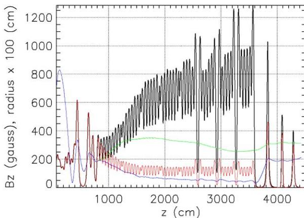
Figure 2: Axial magnetic fields and beam edge radius for the LPE nominal tune (black and blue, respectively) and a magnetic field reduced by 5 (red and green, respectively)
