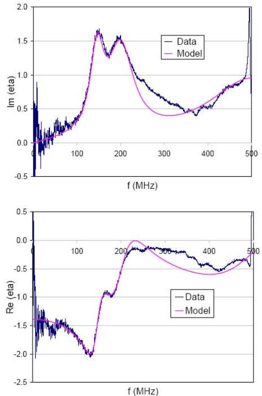
Figure 1: Transverse impedance for DARHT-2 injector cells. The experimental data and the symmetrized model are in blue and pink, respectively.
