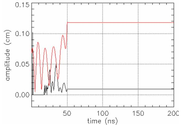
Figure 5: Beam centroid at gap 56 using gap image displacement impedance only, for the nominal case (black) and the reduced  $B_z$  (red).
