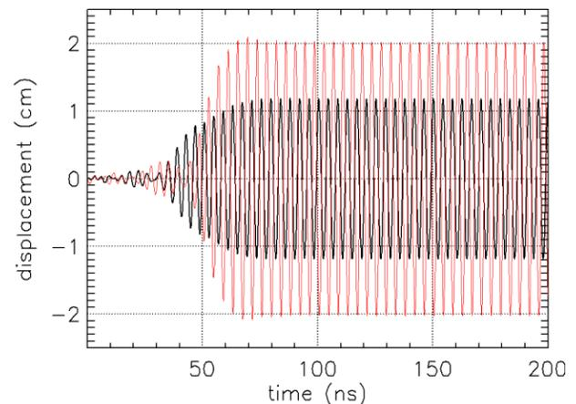
Figure 3: Beam x, y centroid positions (black and red respectively) after 56 cells with an initial 0.1 mm excitation at  $f= 236$  MHz for the reduced  $B_z$  case.
