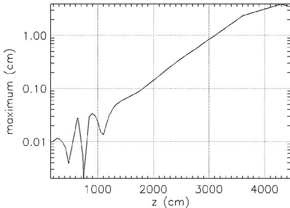
Figure 4: The maximum amplitude of the centroid vs.  $z$  for excitation at  $f=236\text{MHz}$ , showing that BBU grows exponentially with distance (slope  $=1.75 \times 10^{-3} \text{ cm}^{-1}$ ).
