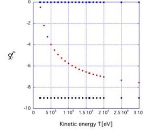
Figure 2: The behavior of chromaticity,  $\xi_{QH}$  for each operation. Red points represent the case that chromaticity is corrected by dc power supply on. Blue points do the case that it is fully corrected. Black points do the case that it is not corrected at all.
