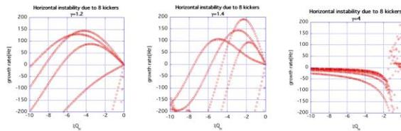
Figure 3: The growth rate due to 8 extraction kickers. The left figure shows the situation at the injection energy. The right figure does at the extraction energy (The growth rate is 0.00028Hz at  $\xi_{QH}=0$ ). The middle figure does at  $\gamma=1.4$ .
